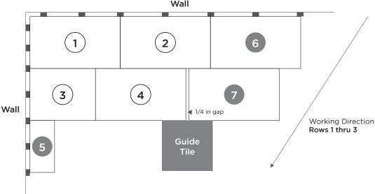
Fig. 2: Work in a diagonal pattern for the first 3 rows.
